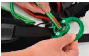
1E: Introduce the unknotted ends of the first rope bridge from inside to outside through the elliptical holes of both front D rings.
