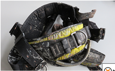
• Traces of paint
