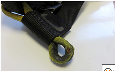
• Damaged attachment point
