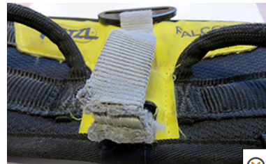
• Damaged attachment point
